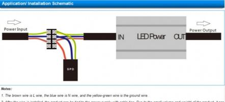
2. After the wire is installed, the product can be tied to the power supply with cable ties. Due to the small volume and weight of the product, it can
